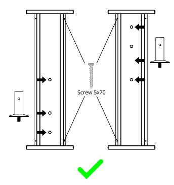
Let footplate be perpendicular to the panel, Recommended to tighten screws for non-slipping and strong wind.
