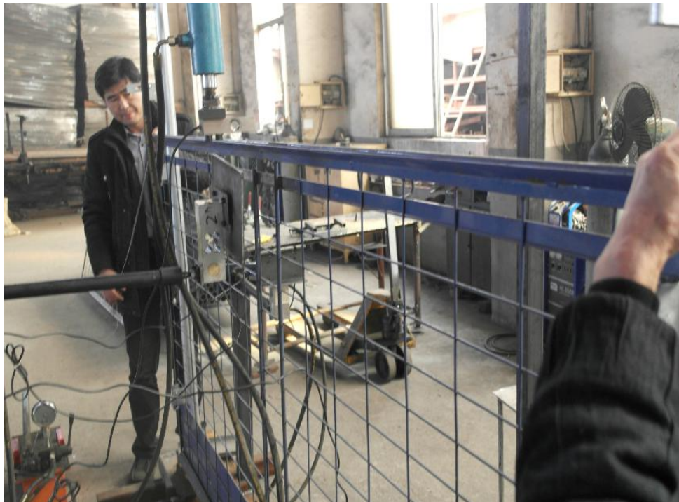
Figure 5, Horizontal loading and deflection measurement
