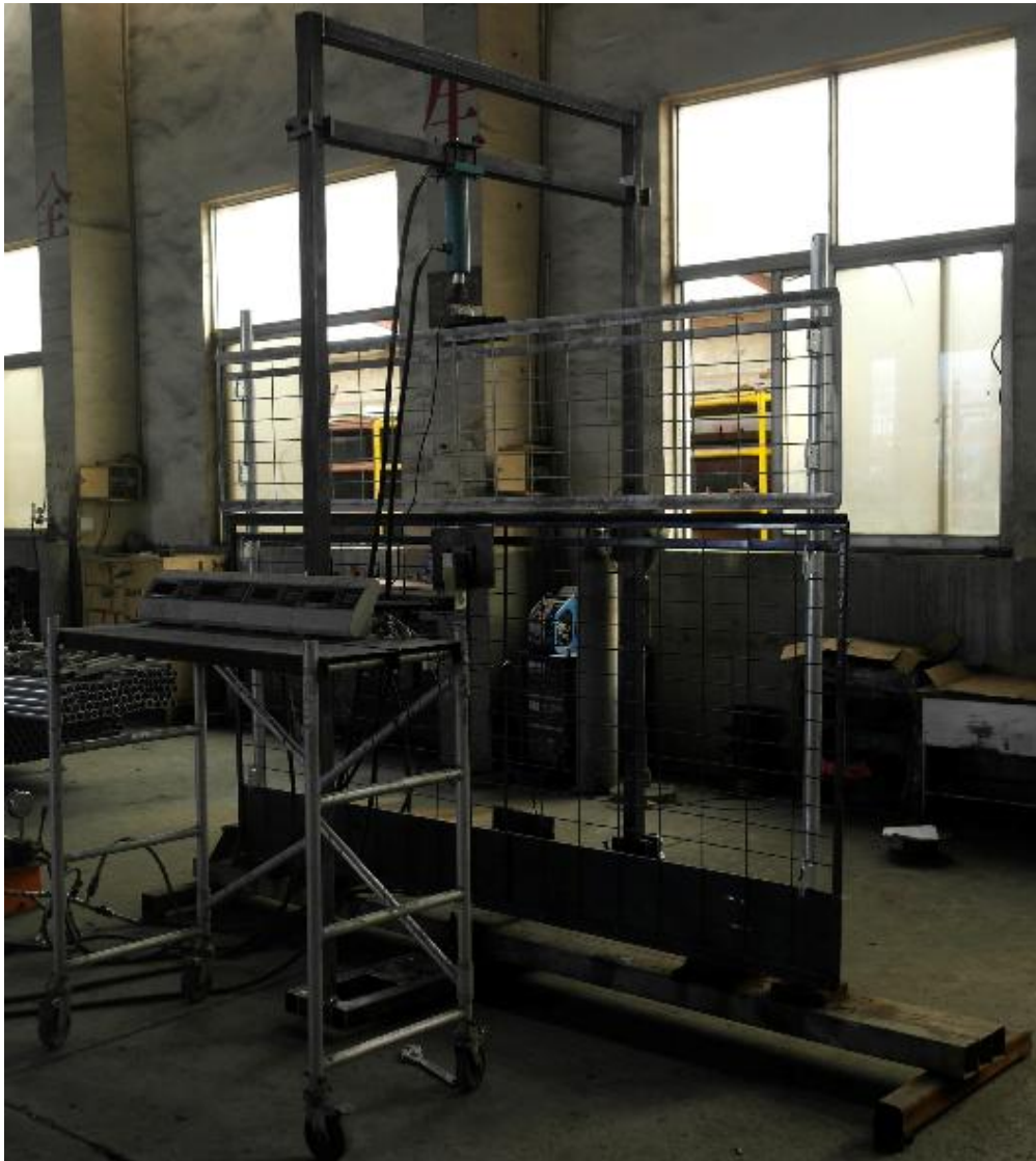
Figure 1, Edge Protection System (King size post with top barrier and bottom barrier)
