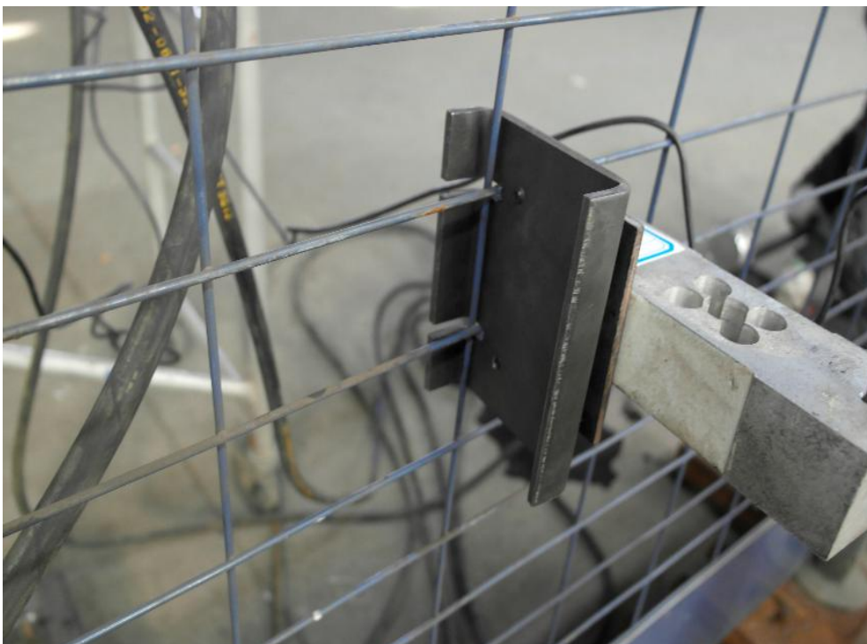
Figure 6, Parallel loading Temporary Edge Protection System Class A Static Tests
