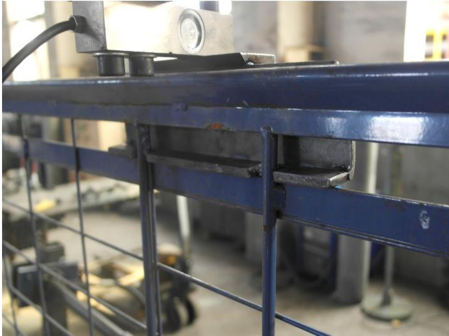
Figure 9, Accidental loading vertical onto mid point
