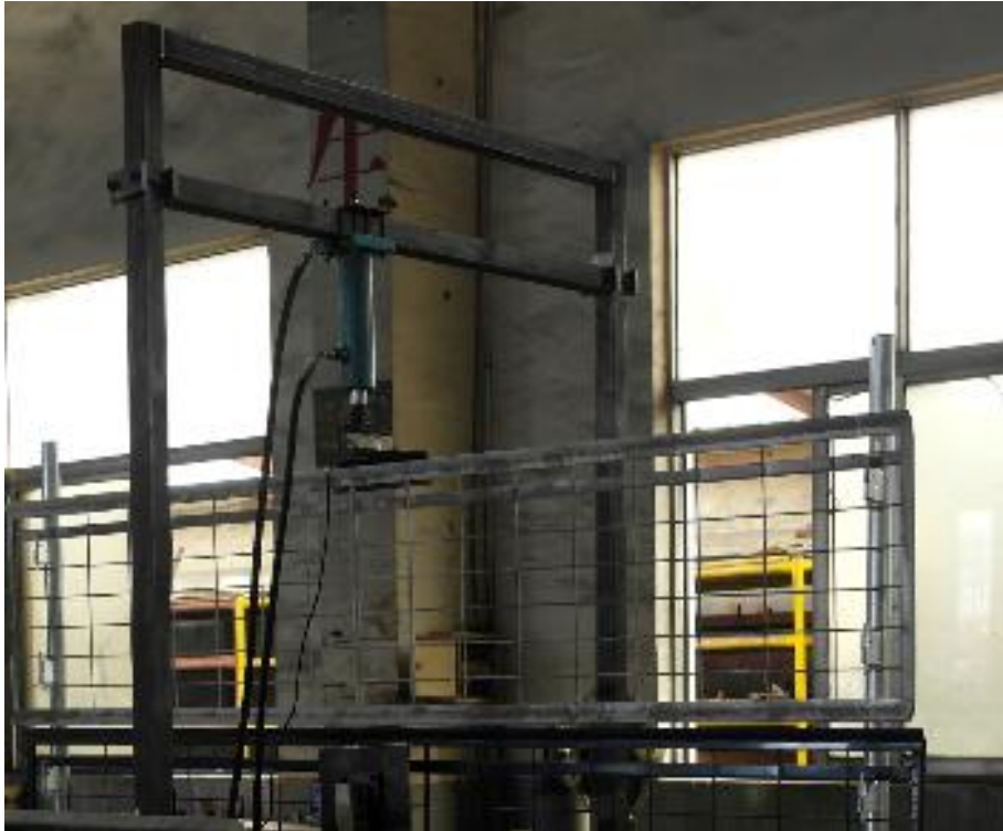
Figure 7, Accidental loading vertical onto mid point
